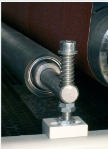
Spring-mounted, rubber coated pressure rollers
