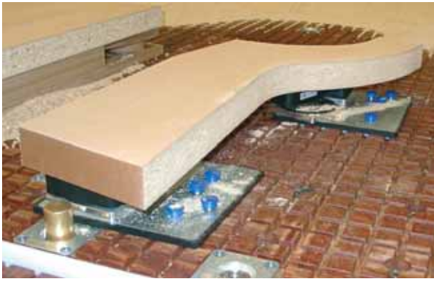
Innospann slotted table suction blocks
